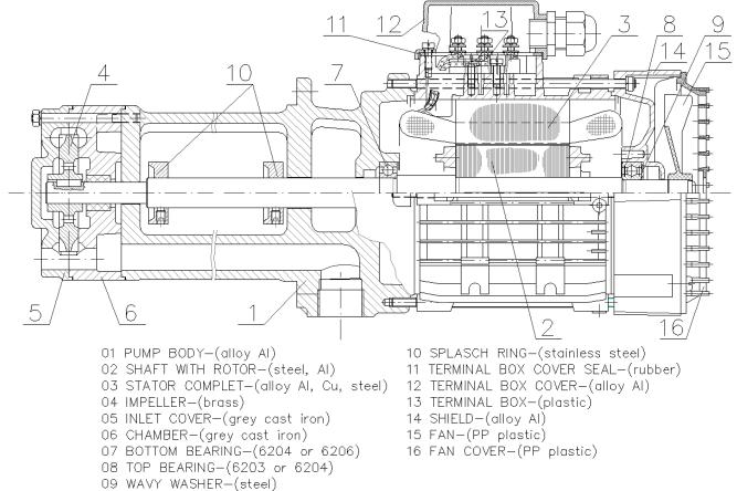
Note: Slide bearings in the hydraulic parts are only machined and molded together with the chamber and form with it a unit *Removal*
